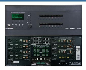
slots, and 2 quad output card slots. Each card slot on the DM-MD8X8-RPS is field-installable, allowing for easy and flexible system configuration with the ability to make changes to the system as needs change.
